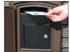
Built-in security insert: Chute drops your mail out of reach of unwanted hands. The mail drops down to a locking rear door for easy collection. The security insert is made of 16-gauge powder coated steel and includes a separate compartment for outgoing mail. The newspaper box is not available with this option. (MAN-LLCOL)
