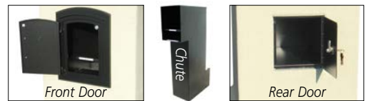
Built-in security insert: Chute drops your mail out of reach of unwanted hands. The mail drops down to a locking rear door for easy collection. The security insert is made of 16-gauge powder coated steel and includes a separate compartment for outgoing mail. The newspaper box is not available with this option. (MAN-LLCOL)
