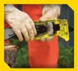
**ATTACH:** When the chain dulls from normal use, dirt contact, or rock strikes, simply attach the bar-mounted sharpener to the PowerSharp<sup>®</sup> guide bar. Twin guide holes in the tip of the bar make perfect alignment foolproof.
