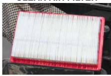
RESTORE AND MAINTAIN POWER AND PERFORMANCE BY REGULARLY CHECKING AND REPLACING THE AIR FILTER.
